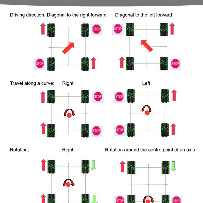
If you require additional directions of movement, you only need to change the direction of rotation of the motors, for instance to rotate anti-clockwise
