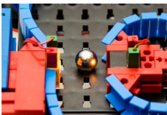
Light barrier for detecting passage
