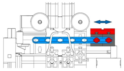
To further reinforce the litter, you can stiffen the strut mount with the following components:
