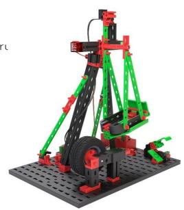
When building the model, make sure that the ship just rests on the tire. Then swing the swing by hand and use the interface test to ensure that the reed contact triggers when the magnet on the ship's swing passes the reed contact.
