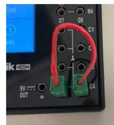
6. After a few seconds, the ON/OFF button should flash alternately red/green. This means that the firmware is being flashed. This usually takes about 5 minutes.
